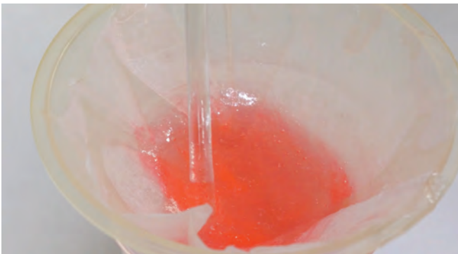
Wax formation in untreated diesel fuel plugs a coffee filter.
