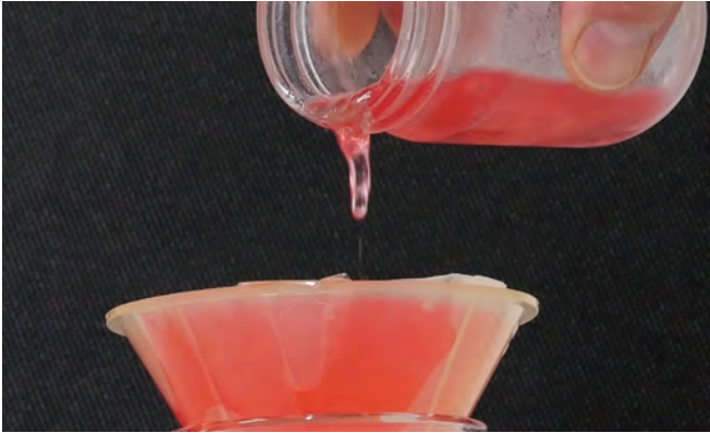
Wax formation in untreated diesel fuel resists pouring.
